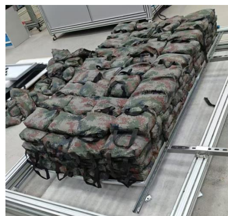
Fig. 10: view of mechanical load mounting
