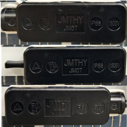
Fig. 5: detail view of closed junction box
